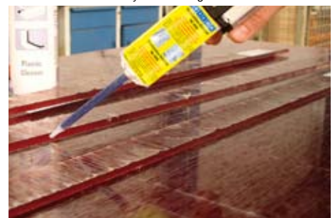
Bonding of various acrylic glass elements for store construction
