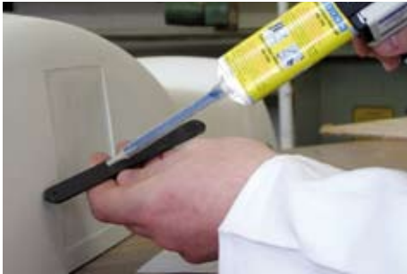
Bonding of metal slats to a protective covering made of polyester for agricultural machines
