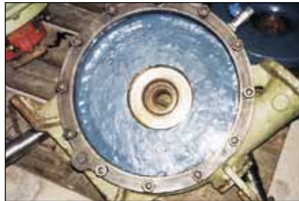
WEICON Keramik BL - Coating of a pump case
