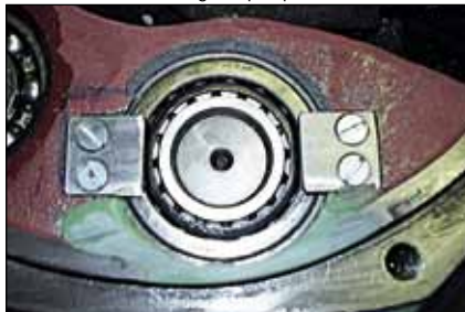
Epoxy Resin Putty - Repair of a gearbox
