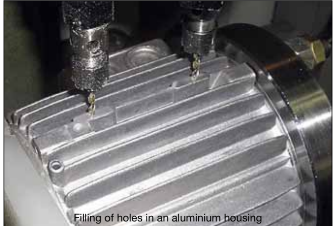
Filling of holes in an aluminium housing
