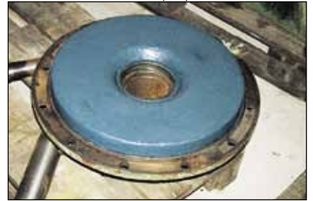
WEICON Ceramic BL - Coating of a pump case lid
