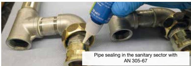
Sealing of a threaded drinking water pipe with AN 301-65
